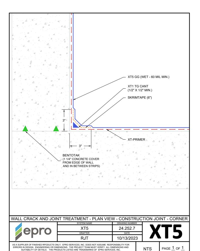
\shortcut-largets-by-id/0B1j3RtmQZ-biQUNqNGJPcEc021kEpro Master FolderDrafting/Details/Walls/XT5/24.252.7 WALL CRACK AND JOINT TREATMENT - PLAN VIEW - CONSTRUCTION JOINT - STATIC dwg [Detail] October 13, 2023 - 2.00pm
