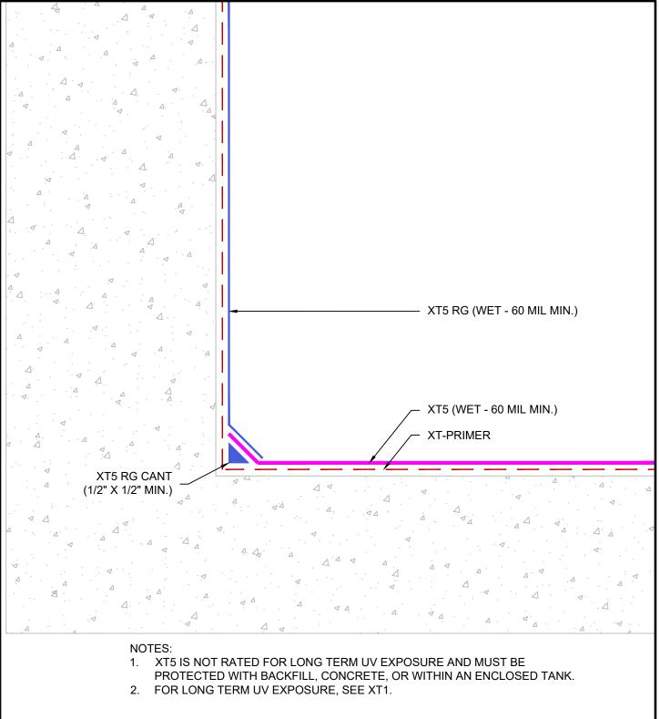
G:\.shortcut-targets-by-id\0B1j3RtmQZ-btQUNqNGJPcEc0Z1k\Epro Master Folder\Drafting\Details\Decks\XT5\24.440.2.1 DECK ASSEMBLY - VERTICAL TRANSITION WITHOUT CONSTRUCTION JOINT - UNREINFORCED.dwg [Detail] September 19, 2022 - 4:10pm
