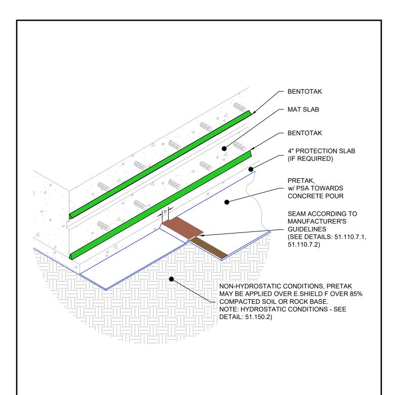
G:\My Drive\Epro Master Folder\Drafting\Details\Underslab\Pretak\51.150.1 UNDERSLAB ASSEMBLY - ISOMETRIC - WITH COMPACTEDSOIL BASE & PROTECTION SLAB.dwg [Detail] April 12, 2021 - 1:03pm
