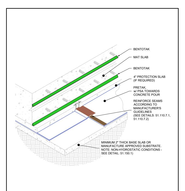
G:\My Drive\Epro Master Folder\Drafting\Details\Underslab\Pretak\51.150.2 UNDERSLAB ASSEMBLY - ISOMETRIC - WITH BASE & PROTECTION SLAB.dwg [Detail] April 12, 2021 - 1:02pm
