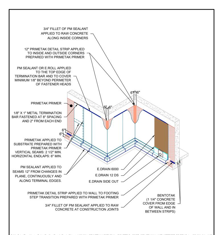
G:\My Drive\Epro Master Folder\Drafting\Details\Decks\Primetak\55.800.1 PRIMETAK ASSEMBLY - ISOMETRIC - POST-APPLIED WALL WITH STEPPED FOOTING.dwg [55.800.1] April 27, 2021 - 9:07am
